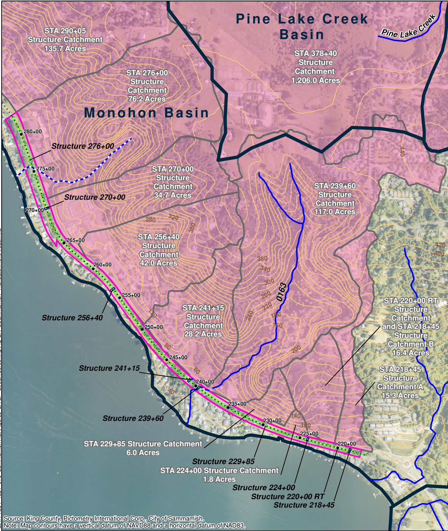
Exhibit 12 Figure 2A SSP 2016-00415 Trail Drainage Structure Catchment Areas
