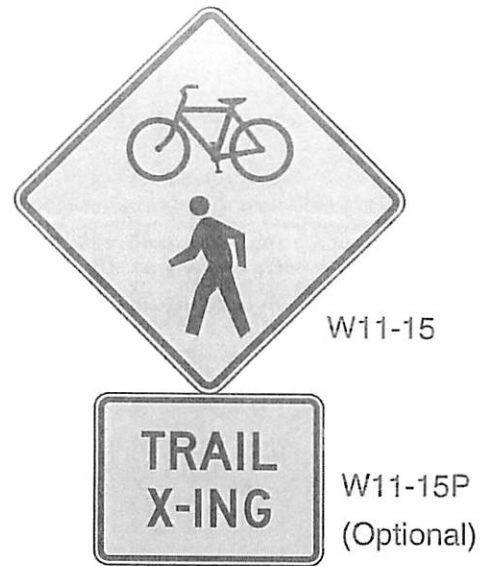
Figure 5-24. Advance Warning Assembly Example
