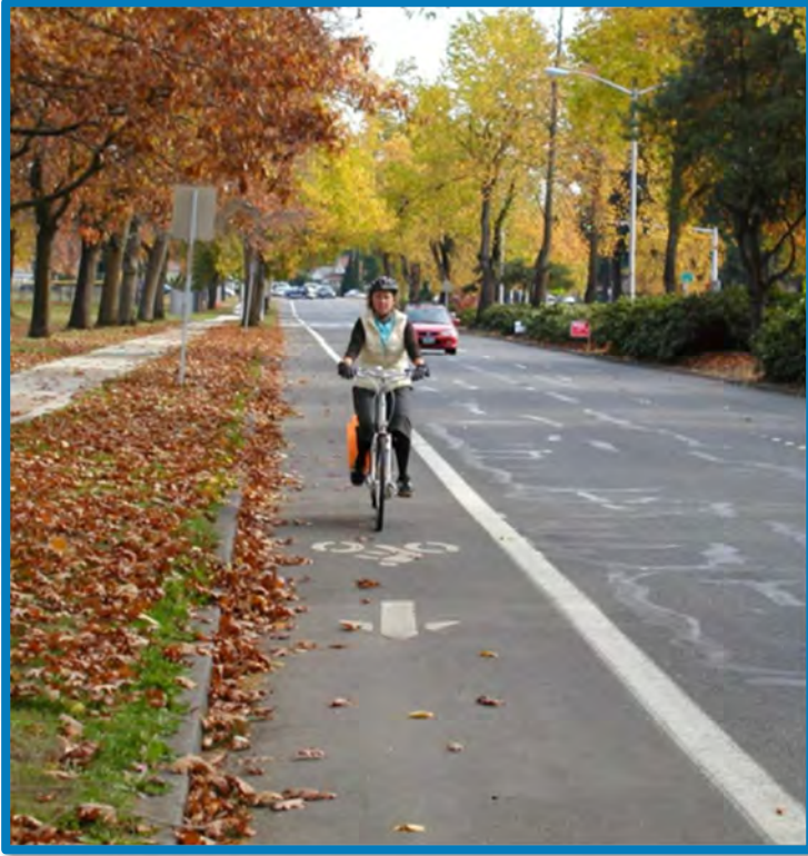
FIGURE 35. CONVENTIONAL BIKE LANE (SOURCE: WSDOT)
