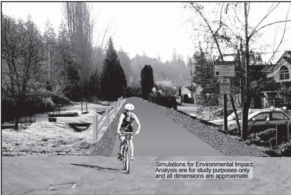
Corridor Alternative; Looking south from railbed at Mint Grove entrance. Paved path is 12 ft. wide with 2 ft. gravel shoulder on left and 5 ft. equestrian path on right.
